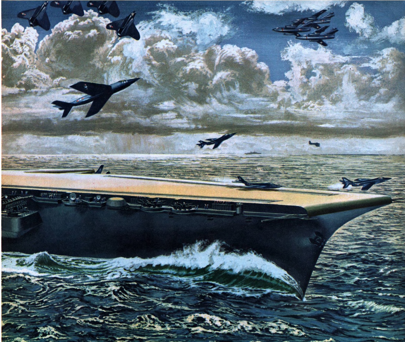
from its unobstructed deck. Ship will be over 1,000 feet long, displace more than 60,000 tons, carry some 3,000 men, support about 100 planes
